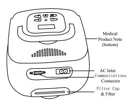
**AC Inlet** ...... Connect/disconnect the AC power cord here.
