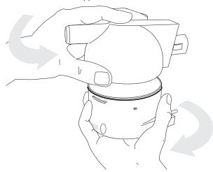
Empty the reservoir and clean it under running water. Remove the lime scale residue from it by wiping it with a soft cloth.
