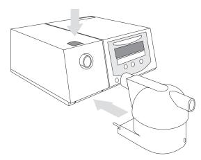
On **AquaTREND III-H5** the heating level is selectable in 6 stages from 0 to 5. By touching the touch pad the heating level will increase at a time for one stage until 5 and then begin with 0.
