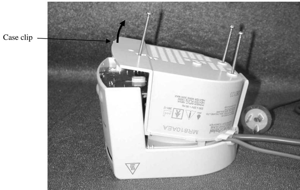
**Figure 6.1: Removing the case bottom**
